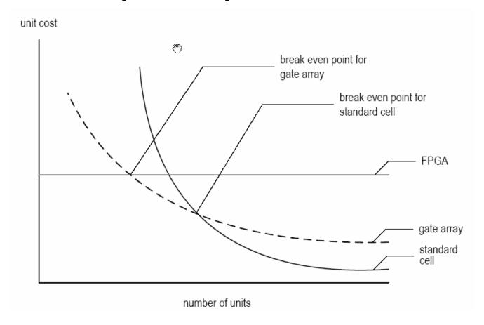
$$C_{per\_unit} = C_{per\_part} + \frac{C_{nre}}{\text{units produced}}$$
