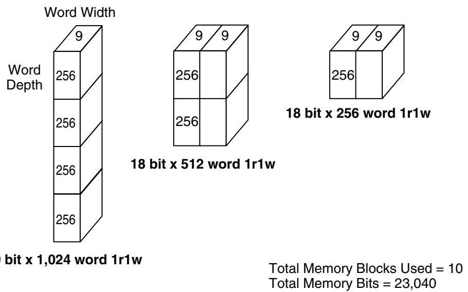
**Figure 13 • Example Showing Memories with Different Width and Depth**
