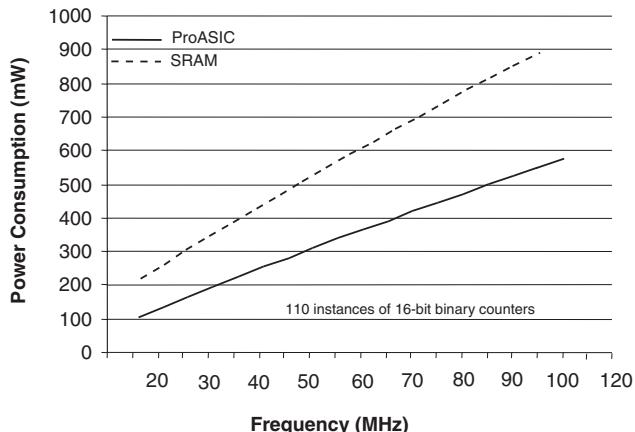
**Figure 16 • Power Consumption of a 500K Device**
