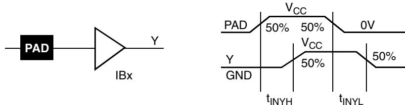
**Figure 19 • Input Buffer Delays****Table 5 • Input Buffer Delays**(Worst-Case Commercial Conditions,  $V_{DDP} = 3.0V$ ,  $V_{DDL} = 2.3V$ ,  $T_J = 70^{\circ}C$ )
