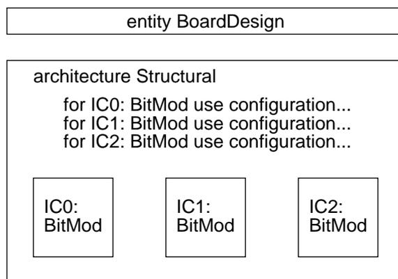
**Figure 10:** *Board design architecture with configuration specifications.*
