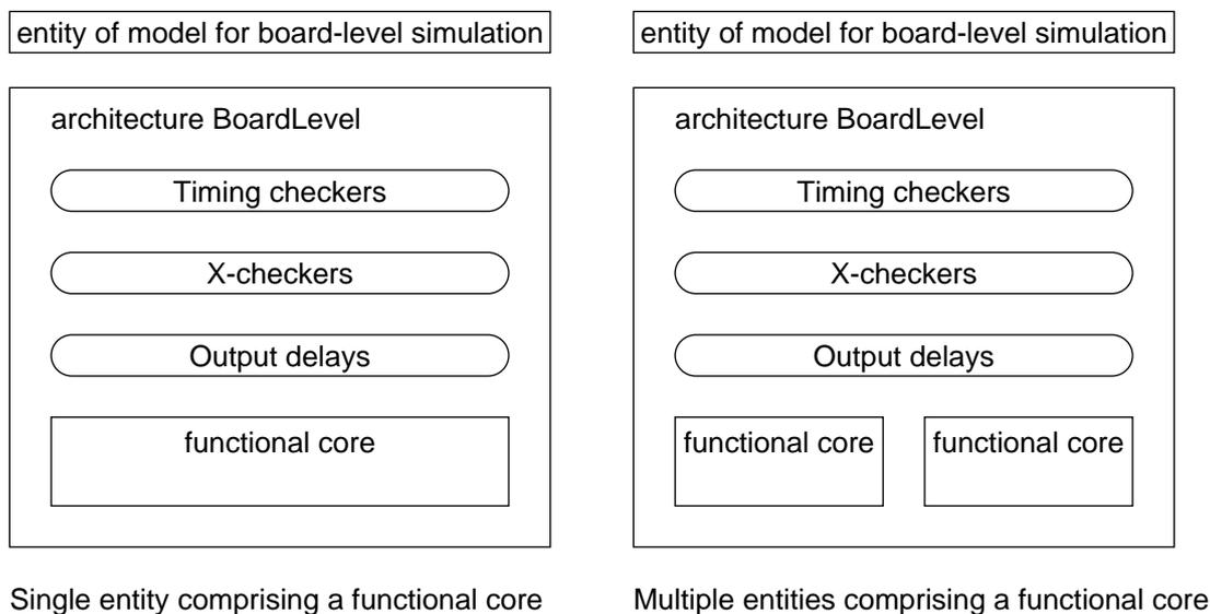
**Figure 2:** Preferred two-level hierarchies (squares with rounded corners are processes or concurrent procedures, regular squares are subcomponents).
