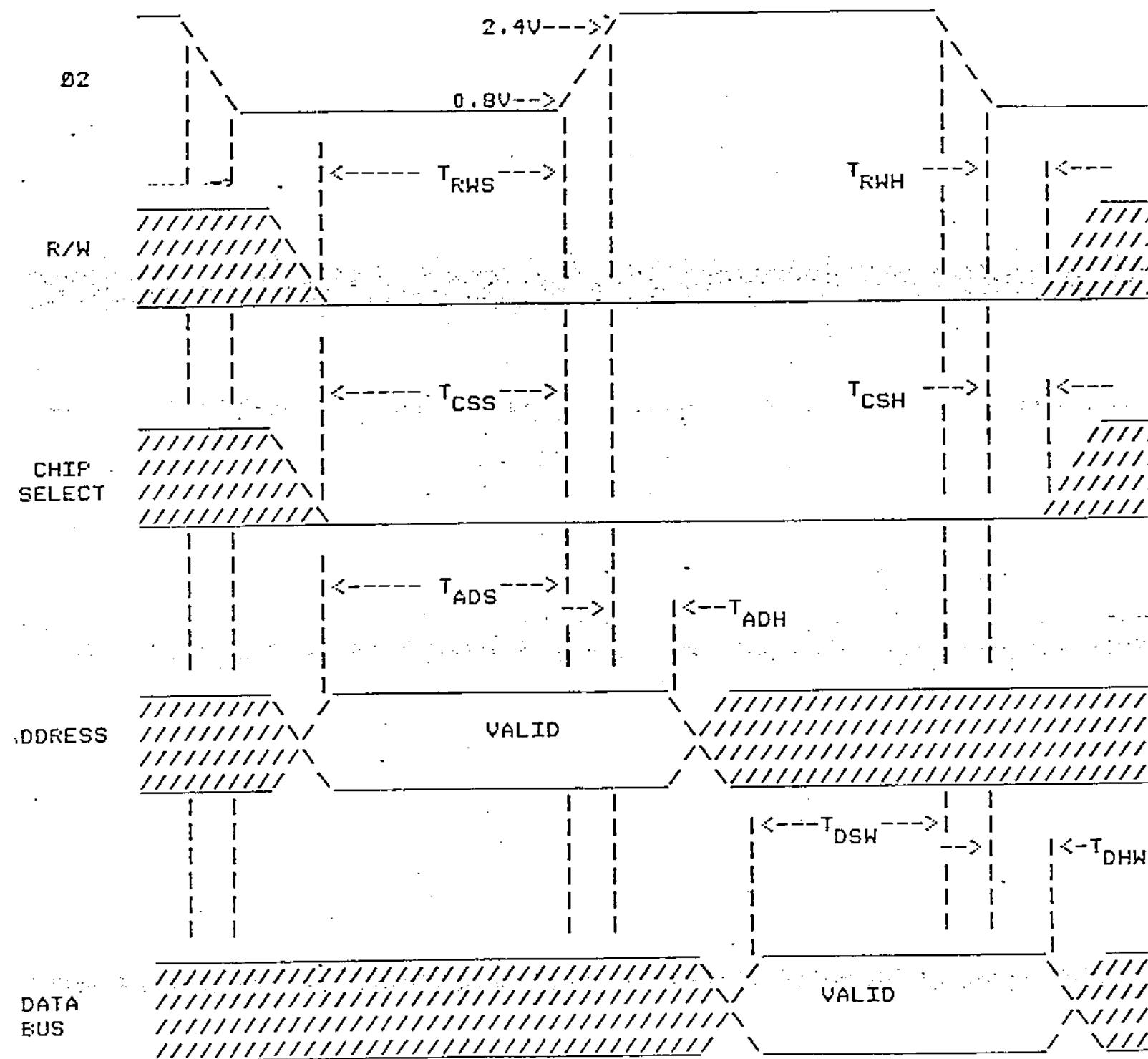
NOTE: ADDRESSES ARE CLOCKED IN ON THE LEADING EDGE OF  $\overline{Q2}$ .
