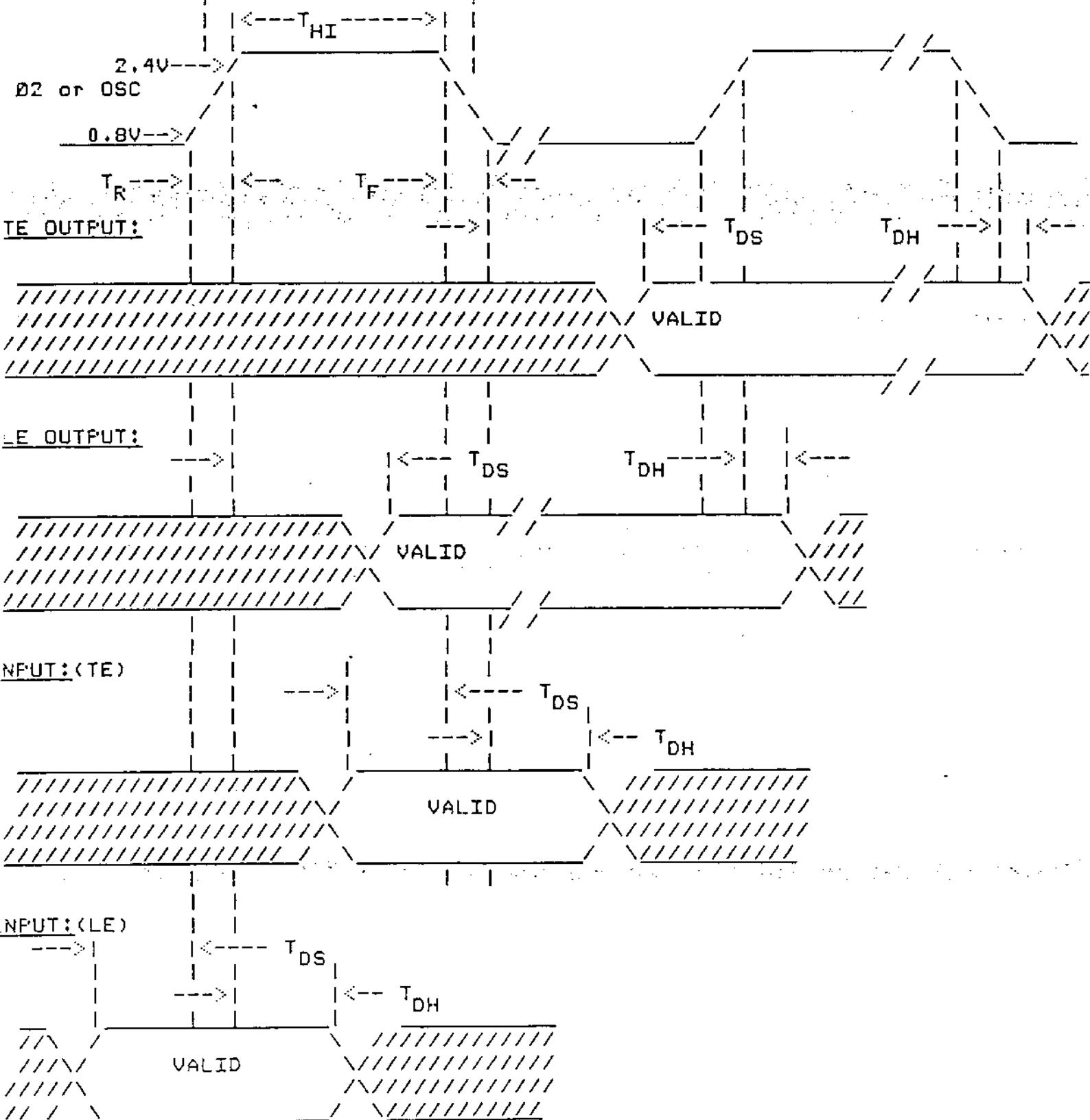
1.5) WRITE I/O TIMING: (MICROPROCESSOR WRITING TO THE GTIA)
